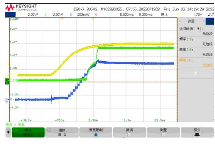
VINP =5V(黄色), VISO=5V(绿色), 软启动波形, IISO=300mA(蓝色)
